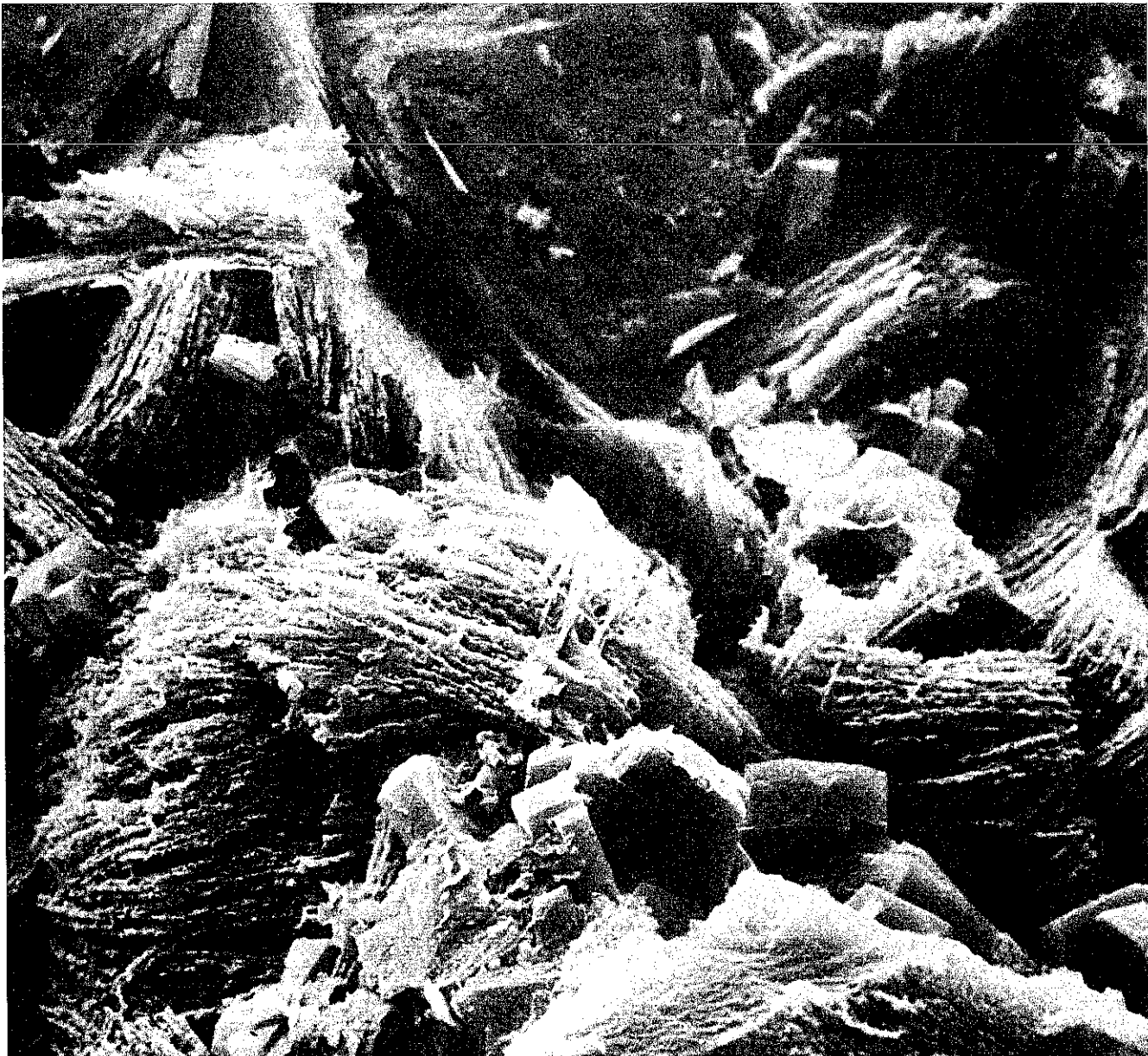
Figure 2. Chabazite (long chains of individual crystals) approximately 0.2 microns in size and clinoptilolite (larger coffin-shaped crystals) from the Bowie chabazite deposit.
